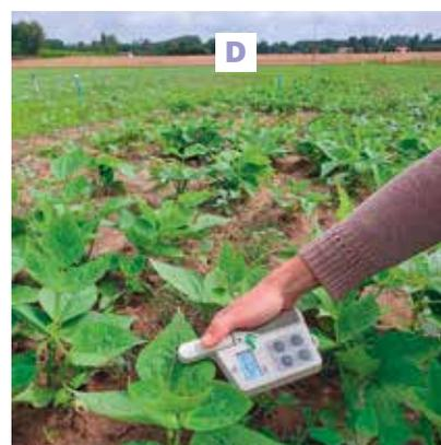
> OUTILS DE DIAGNOSTICS POUR ÉVALUER LA TENEUR EN AZOTE DES CULTURES : (A) DUALIX (FORCE-A), (B) MULTIPLEX (FORCE-A), (C) POLYPEN (PHOTON SYSTEMS INSTRUMENTS) ET (D) SPAD-502 (KONICA MINOLTA). CES APPAREILS PERMETTENT LA MESURE D'INDICATEURS PHYSIOLOGIQUES DE LA PLANTE POUVANT ÊTRE RELIÉS AU STATUT AZOTÉ DE LA PLANTE.
